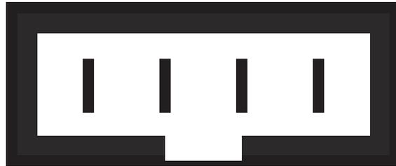
Figure 4-3: J4 - RS-232 Jack Pinout
