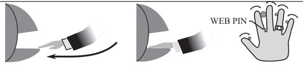
Figure 8-2: Placing Your Hand on the Platen
